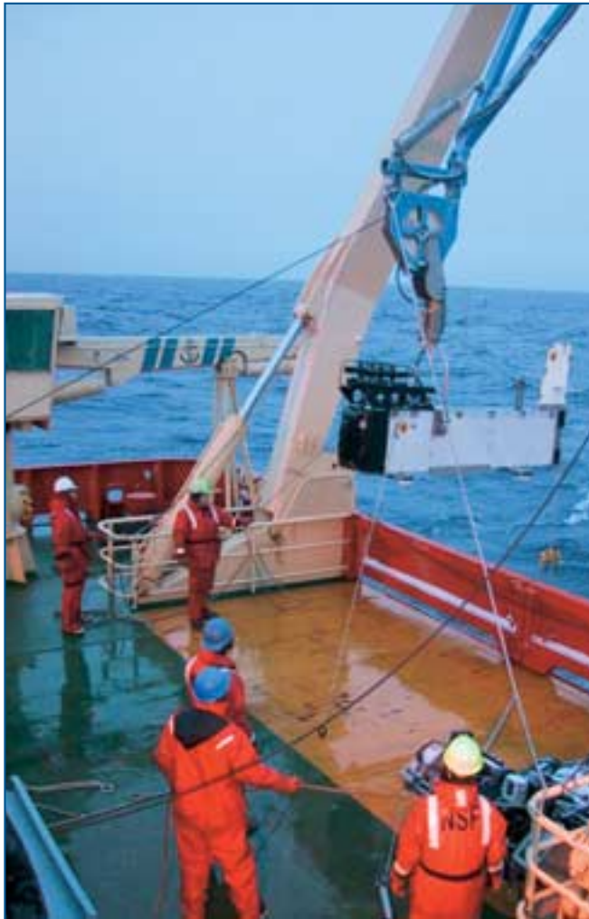
Figure 3. The Bio-Optical Multifrequency Acoustical and Physical Environmental Recorder (BIOMAPER-II) being brought back on board the RVIB Nathaniel B. Palmer during the first U.S. SO GLOBEC survey cruise, 17 April to 5 June 2001. Photograph by Eileen Hofmann.
