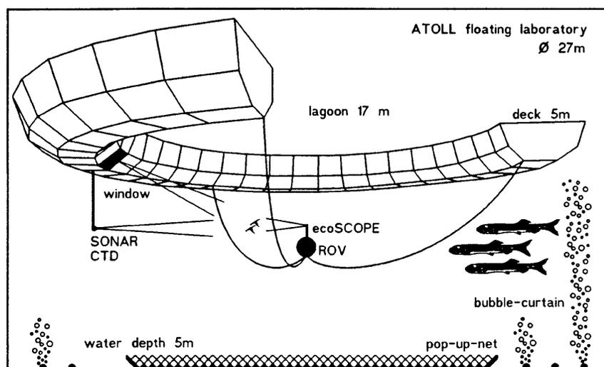
Figure 1. The ATOLL floating laboratory showing tethered ROV with attached ecoSCOPE.
